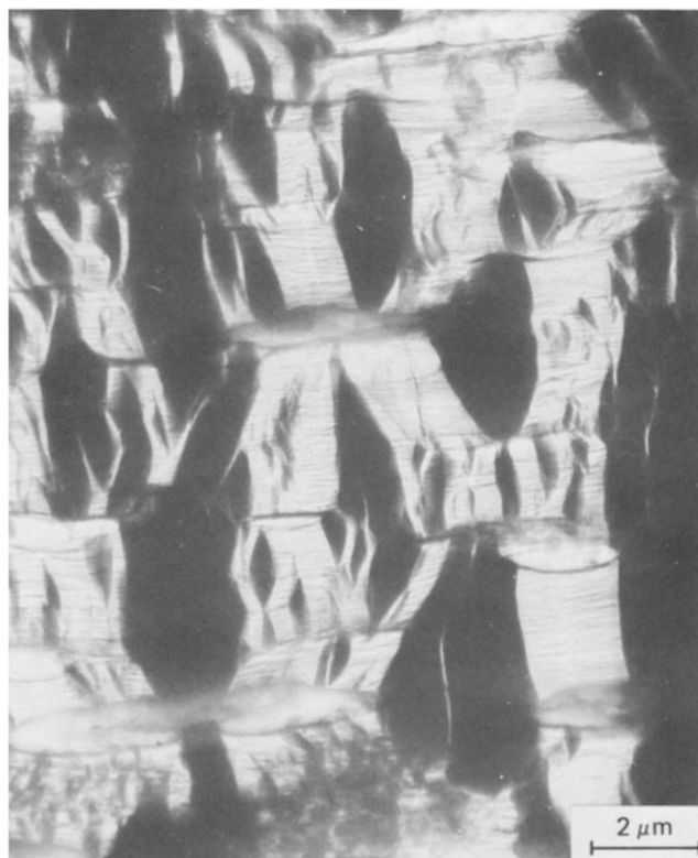
Figure 7 Formation of broad long-craze-bands in HIPS due to the superposition of stress fields (deformation direction horizontal)
